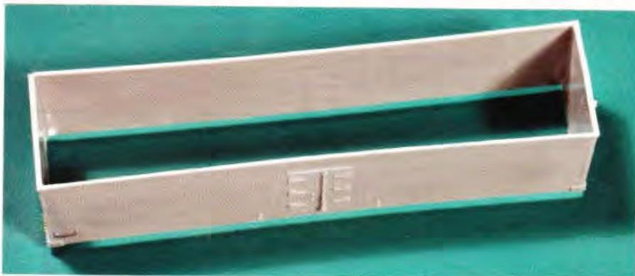
The sides and ends of this refrigerator car kit (*above*) have been glued together. Although the sides of resin kits can sometimes be slightly warped, the sides on this refrigerator car are just flexible because they are thin. The basic carbody (*below*) is seen with a pair of floor spacers clamped in place. The body is right side up with the floor below it.
