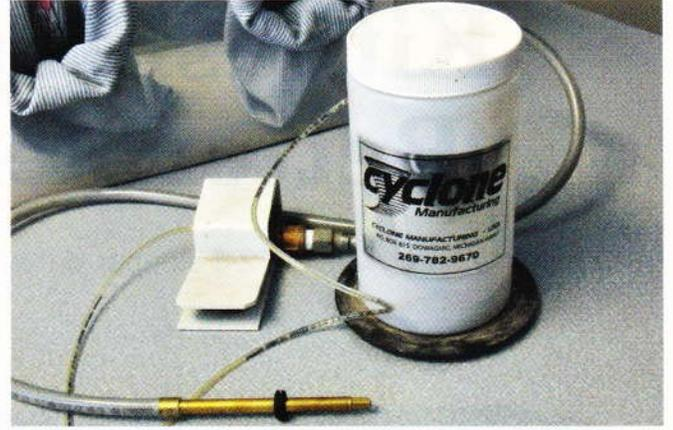
(above right) are the shop vacuum connection, a pencil sandblaster, a container of abrasive and a foot pedal air valve.
