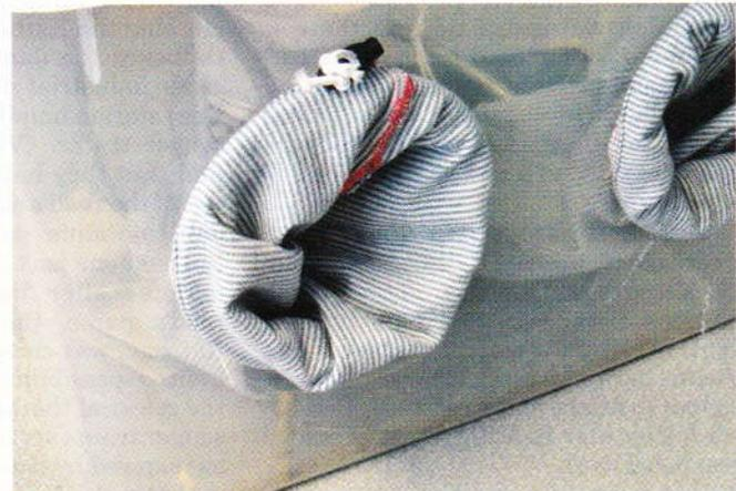
The sandblasting booth (top) was easy to build from a plastic storage box. A hole was cut and fitted (above left) with a piece of clear acrylic so one can see into the box during use. Note the
